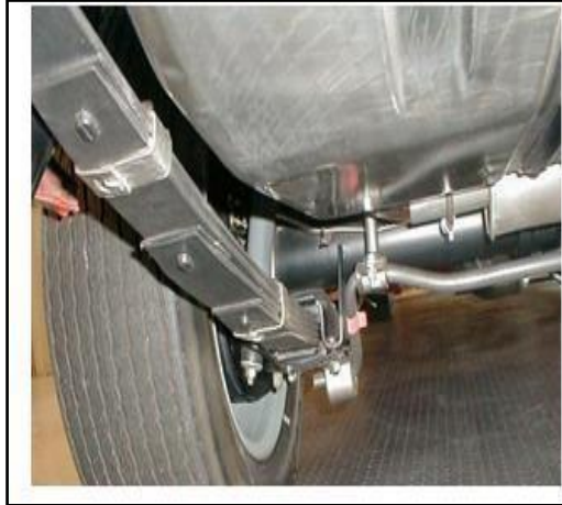
Fig. 1 A Traditional Leaf Spring Arrangement
