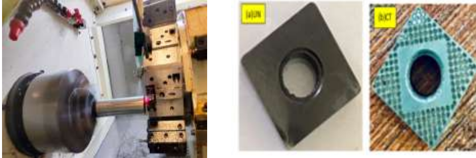
Figure 1. Schematic view of (a) untextured tool (UN) and (b) circular pit hole texture (CT).
