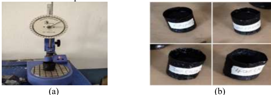
Figure 4: (a) Penetration Test (b) Penetrometer and Canisters containing CRMB samples with varying Crumb Rubber proportion
