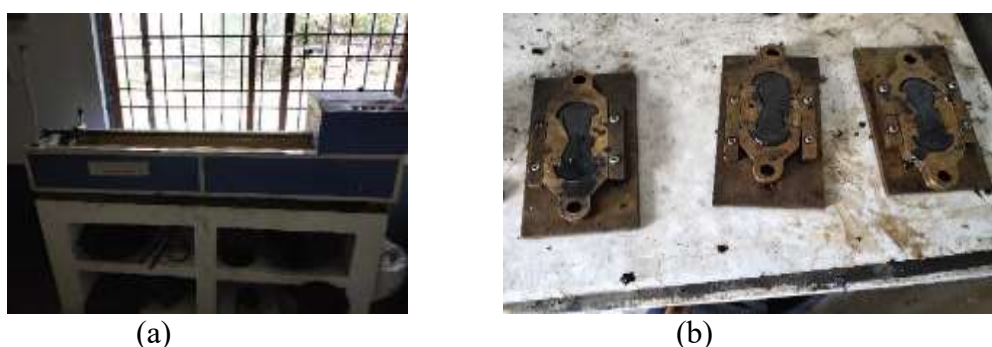
Figure 3: (a) Ductility testing machine (b) Brass Ductility Moulds used for Ductility Test.
