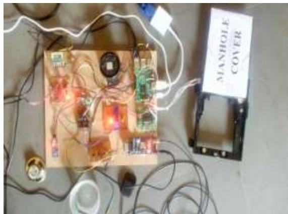
Figure 7(b): Manhole cover opened when water level crossed the cutoff level
