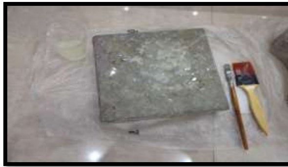
Fig- 6- Coat on surface of Paver Block
