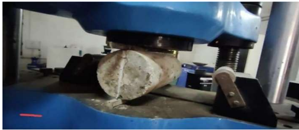
Figure 9 Test setup of split tensile strength
