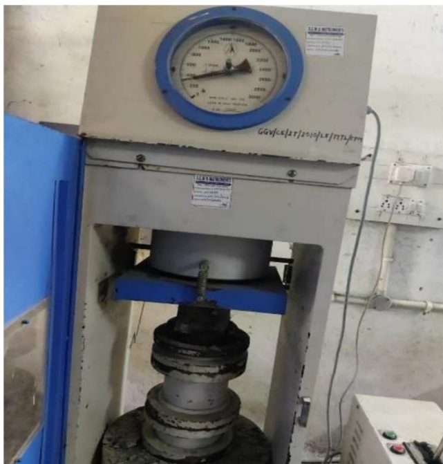
Figure 7 Compressive strength testing of typical concrete samples
