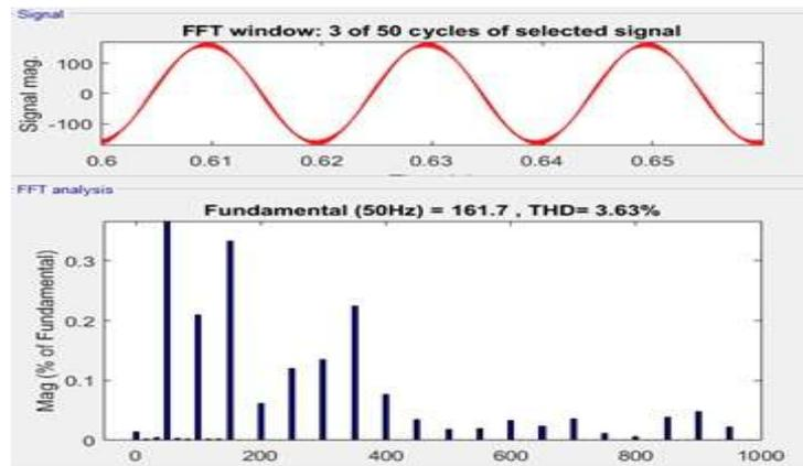
Figure 17: THD of PV inverter current
