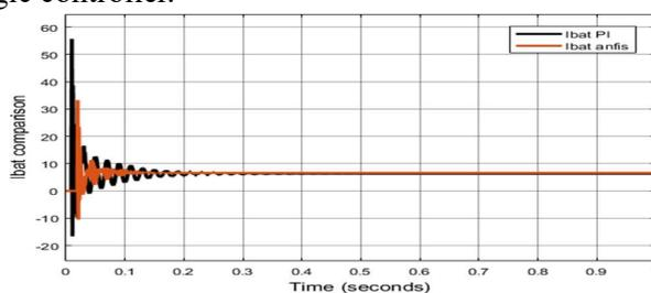
Figure 19: EV battery initial comparison Between PI and Anfis
