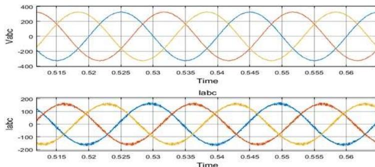
**Figure 13: PV inverter three phase voltages and currents**
