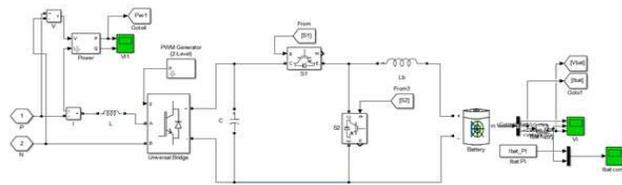
**Figure 10:EV circuit structure with MOSFET Switch**
