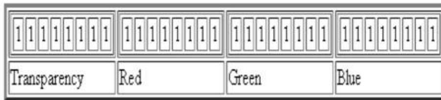
Figure 5: BIT Transferred for Red, Green and Blue plane (24bit=8bit red;8-bit green;8bit blue)
