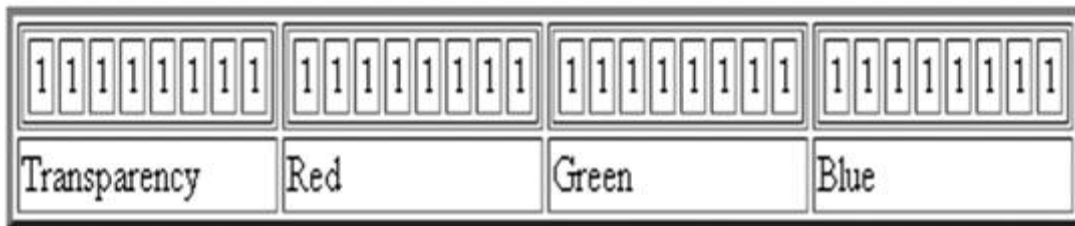
Figure 1: Bit Transferred for Red Green and Blue Plane (24bit=8bit red;8-bit green;8bit blue)
