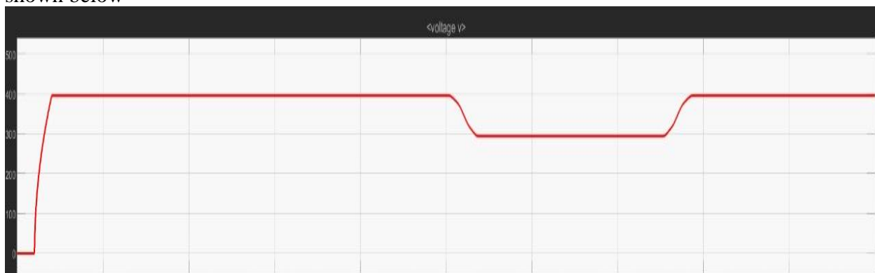
Fig 6.4 Voltage when Fault Resistance is 2
