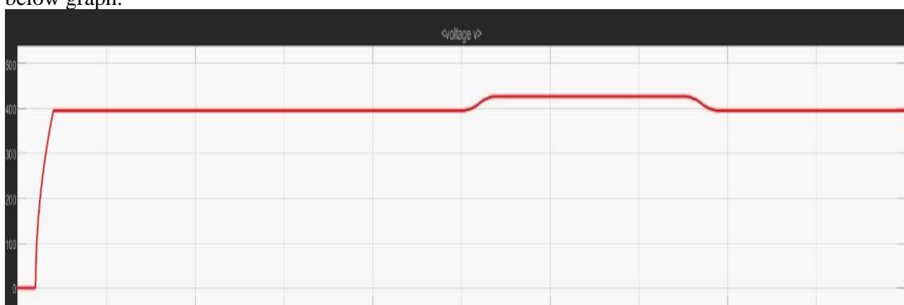
Fig 6.7 Voltage when fault resistance above 6
