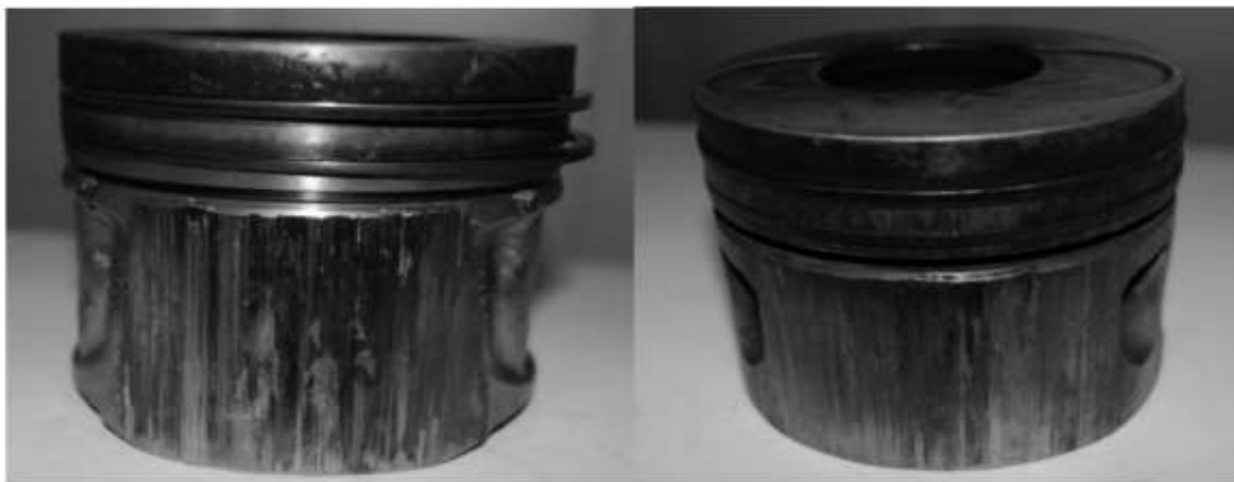
Figure No.4 A Piston Skirt Seizure
