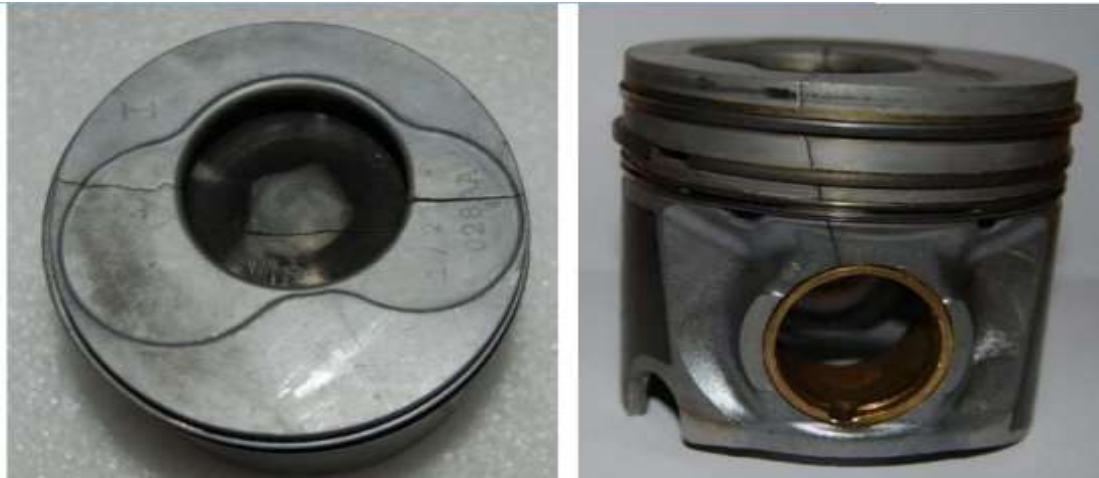
Figure No.5 A Crack On the Piston Pin: A) Cracked Piston Head; B) Cracked Piston Skirt
