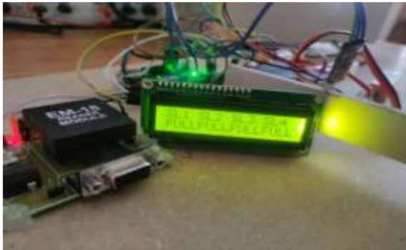
Fig 5.2 LCD Display indicating slot Full after car parking
