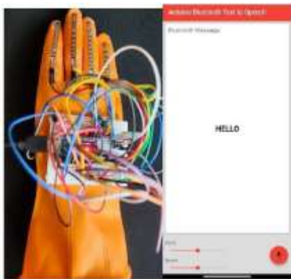
Fig 5.1 Gesture for “HELLO” and the corresponding text is displayed
