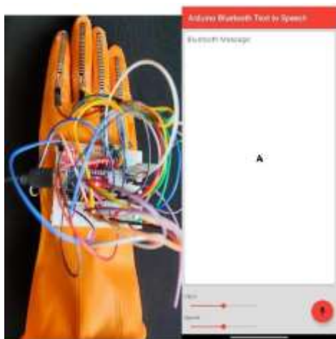
Fig 5.2 Gesture for “A” and the corresponding text is displayed. gesture for “A” and “HELLO” are same but DIP switch 1 and 4 is in on state for HELLO for A 1 and 4 is in off state
