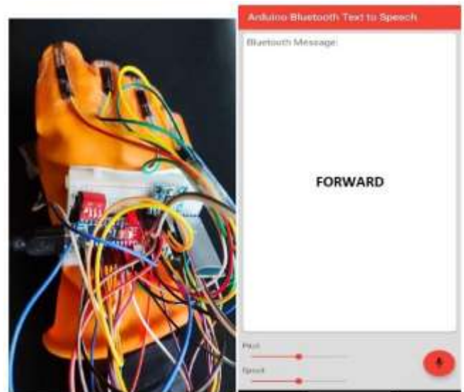
Fig 5.4 Gesture for “FORWARD” and the corresponding text is displayed
