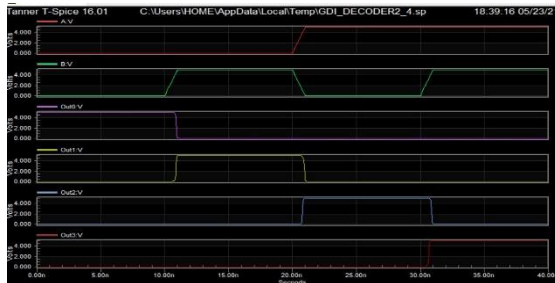
Figure – 4: 2-4 decoder Waveforms
