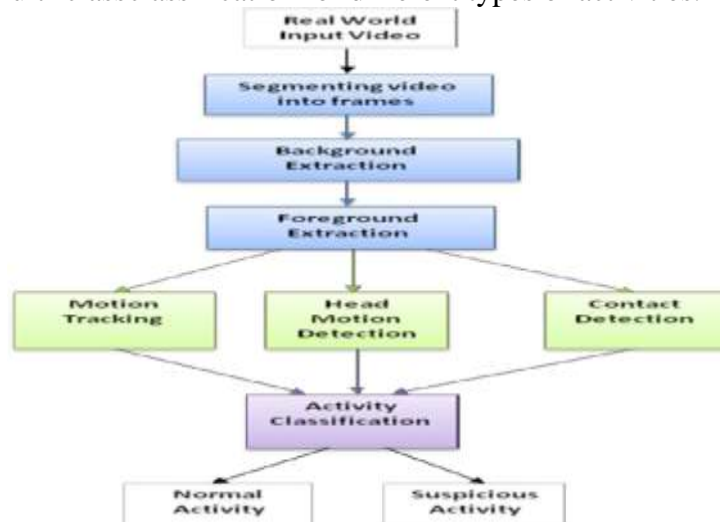
Fig. proposed system showing CNN based feature extraction and tracking of suspicious activity.
