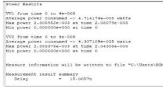
Figure – 6: Existing HP 2-4 decoder power Delay
