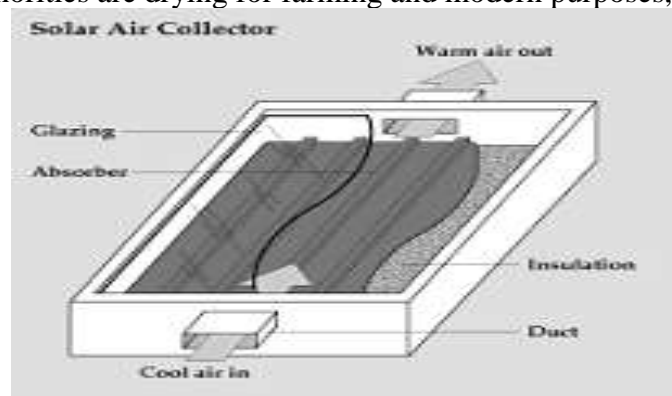
Fig. 4: flat plate air heater collector
