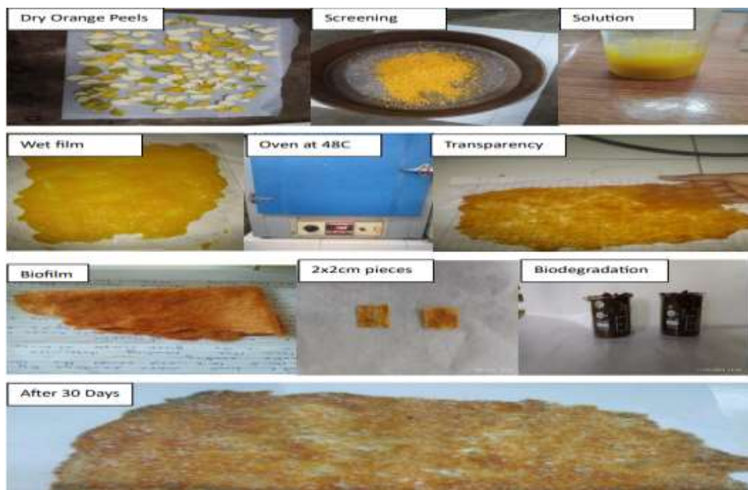
Figure 2. Overall process for orange peels biofilm formation.
