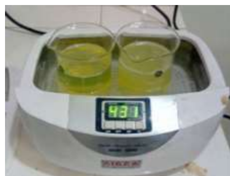
Figure 3.24 Mixture of \text{CeO}_2 & Bio Diesel Blends in Water Bath of Ultra Sonicator
