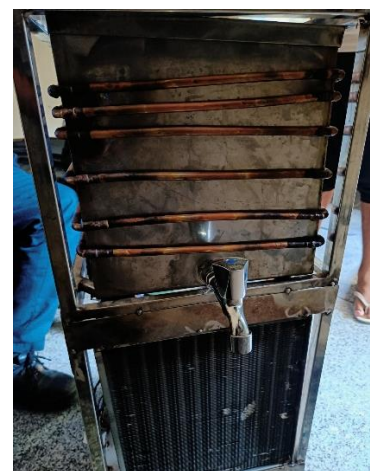
Fig: Working Model of Water cooler working on reversible switch (3-Way valve)
