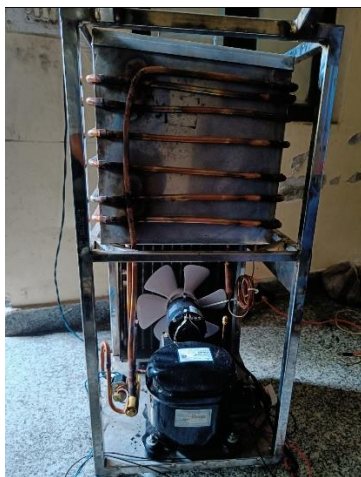
Fig: Working Model of Water cooler working on reversible switch (3-Way valve)
