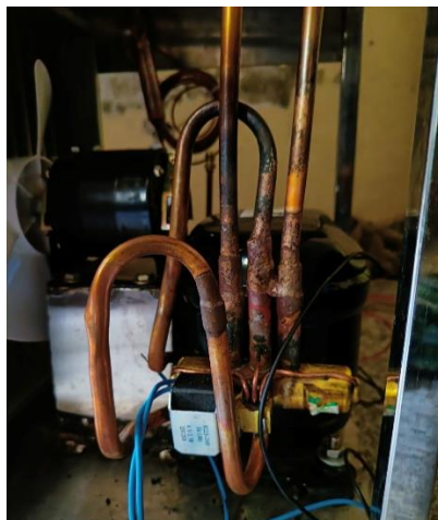
Fig: Working Model of Water cooler working on reversible switch (3-Way valve)
