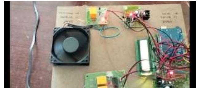
Here Ignition fan is turned ON when the temperature exceeds 33 degrees
