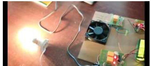
Here, The Bulb will be on when there is an absence of light
