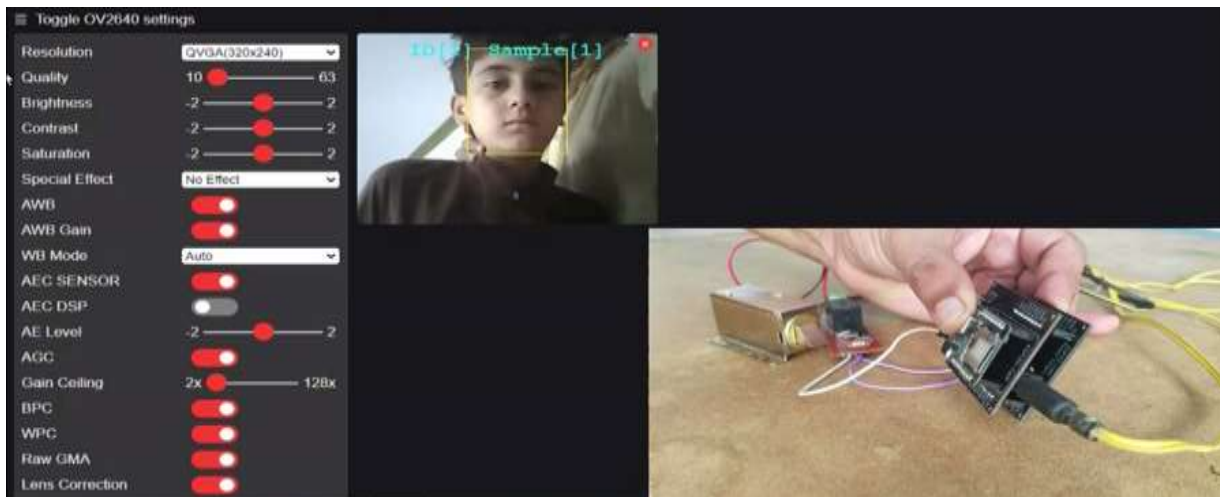
Fig 6:Face detection with the help of Esp 32 cam
