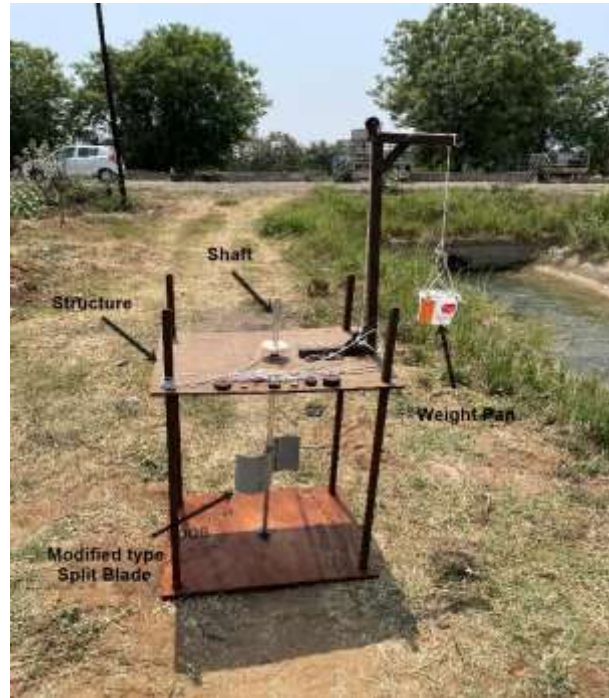
Fig 10. Experimental Setup of Split type Modified Turbine
