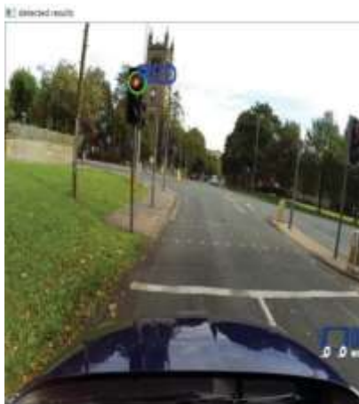
FIGURE 1: The Red Color Traffic Signal is Detected. FIGURE 2: The Yellow Color Traffic Signal is Detected.
