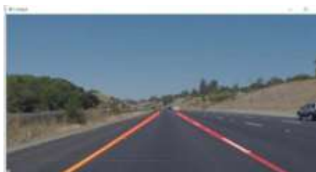
FIGURE 3: The left and Right lanes are detected. FIGURE 4: The Height, Weight, Color of the Hough Line.
