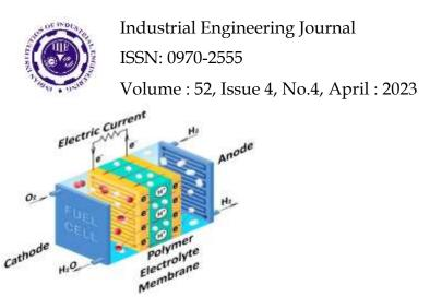
A fuel cell is an electrochemical device that converts chemical energy from a fuel into electrical energy without combustion. Fuel cells use a chemical reaction between a fuel, such as hydrogen or natural gas, and an oxidant, such as oxygen, to produce electricity, water, and heat. Fuel cells are a promising technology for generating electricity because they are highly efficient, clean, and quiet.
