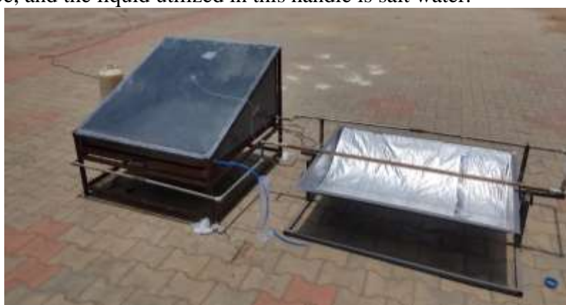
Fig 1: Experimental setup for solar still coupled with PTC
